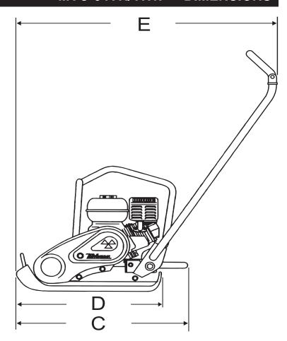
Figure 1. MVC-64VH/VHW Plate Compactor Dimensions
